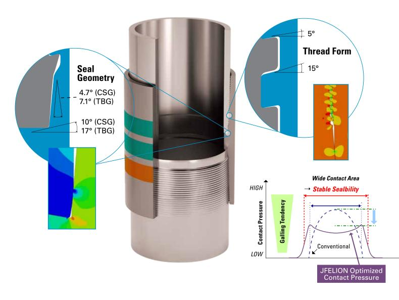
Unique seal profile provides stable contact pressure with low galling risk.
